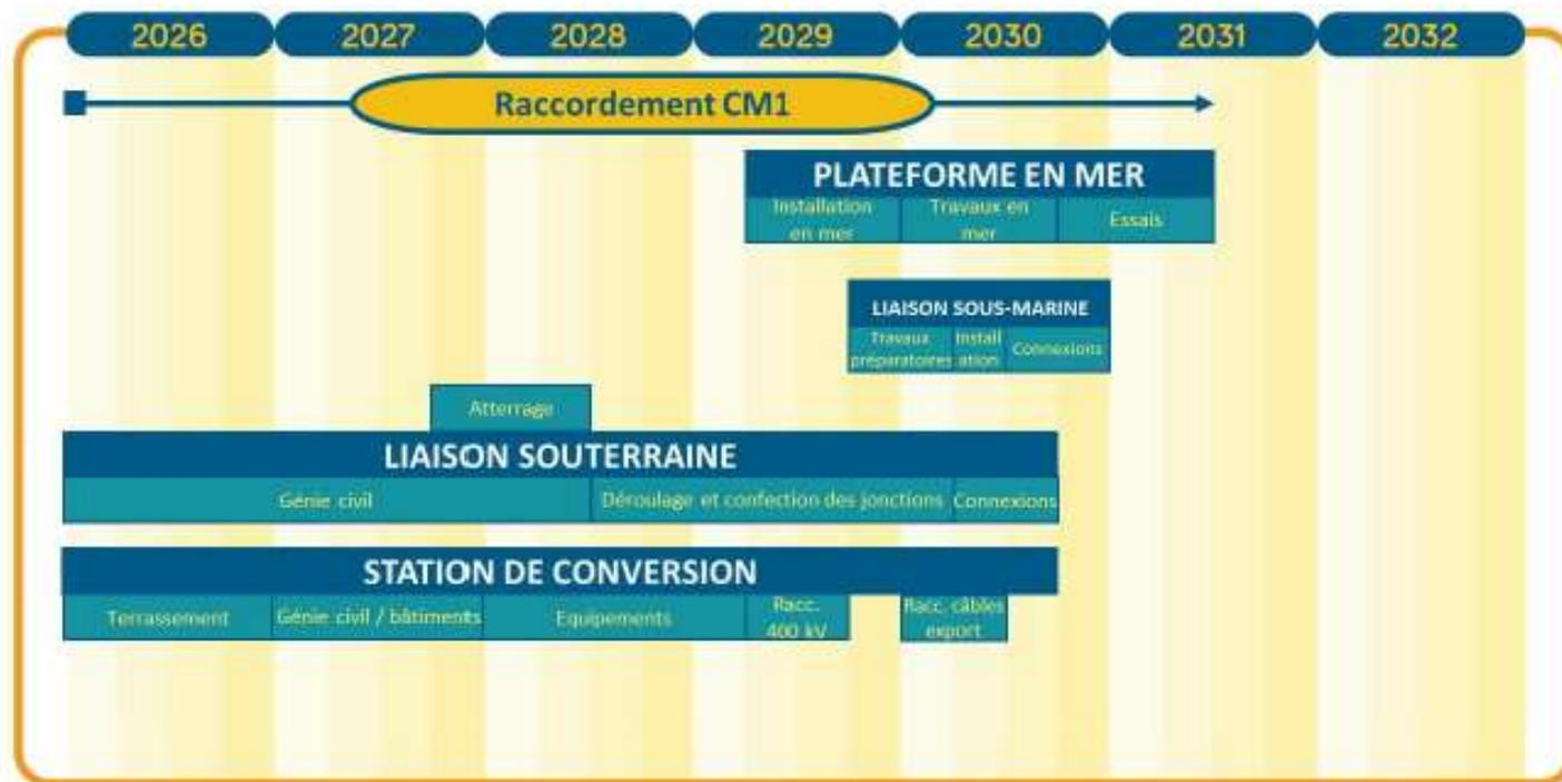
FIGURE 24: PLANNING DE TRAVAUX DU RACCORDEMENT CM1
